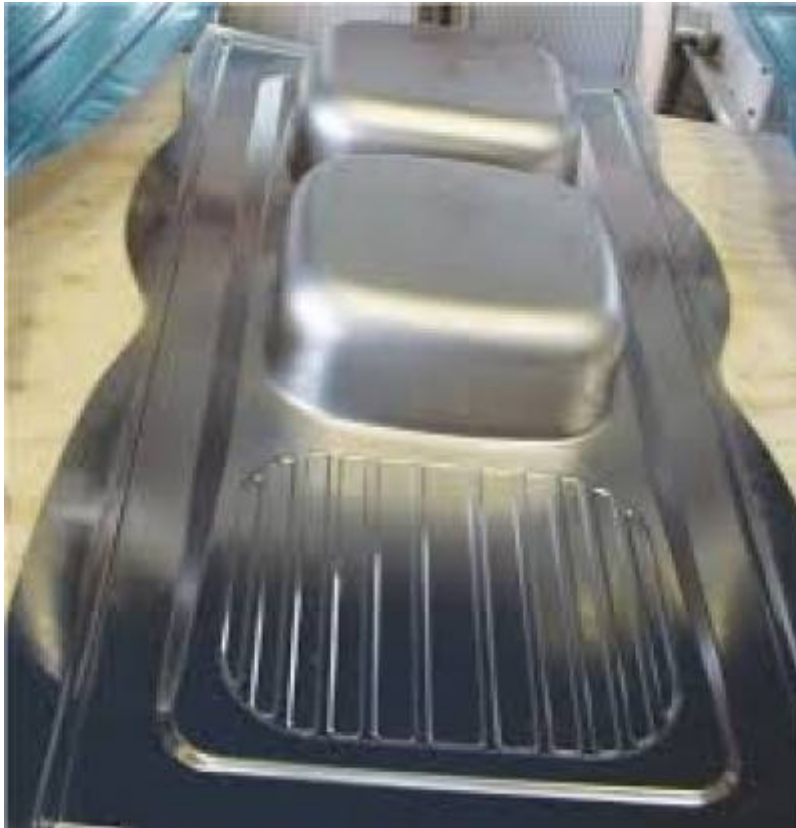
Figure 55: Stamping kitchen sinks
